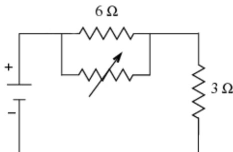
Under what value of the variable resistances given below, power transferred to the fan will be maximum? The power source of the fan is a dc source with internal resistance of 6 ohms.
