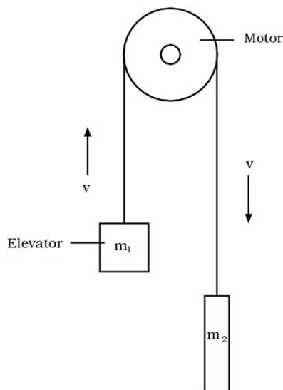
At what rate does the motor provide energy to the system when the elevator is rising at a steady speed  $v$ ? ( $g$  = acceleration of free fall) (consider the pulley as frictionless at the pivot)
